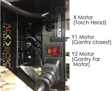
Connect Wire as Shown, Y2 has a different color combination to account for the direction change from Y1
