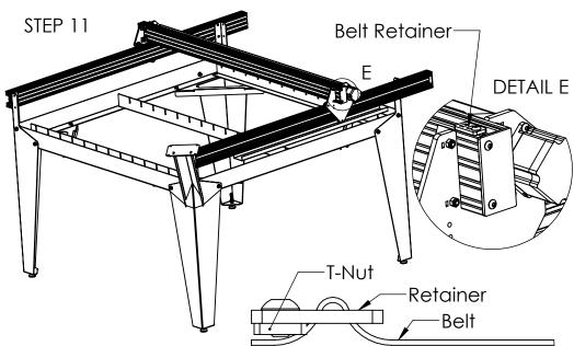
Install Belt Retainer with 10-32x1/4 Capscrew & Tee Nut & End Cap Plate with 10-32x5/8 Capscrew. Belt Threaded through retainer as shown. After install, pull belt retainer to insure a good amount of tension on belt
