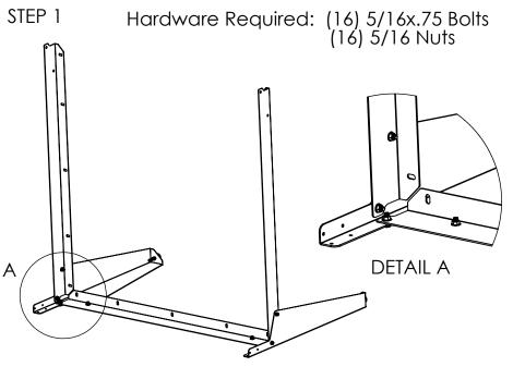
Place legs on floor and bolt frame as shown, leave hardware loose for the next 4 STEPS
