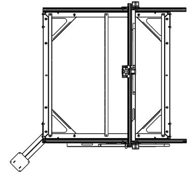
3 Wire Conduit are provided, all 3 must be run thru the lower drag chain, one long must run thru the upper The torch head is considered the X Axis The gantry is considered Y1 & Y2
