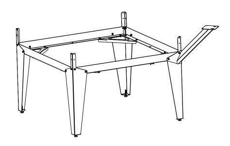
Remove the bolts at any corner while supporting the frame, install Computer Stand using the same bolts removed
