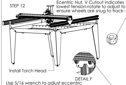
nuts until wheels are snug on V-Slot, remove lower
